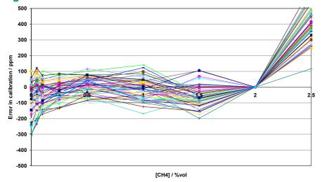
Using universal linearisations, the IRC-AT error is less than 0.05% Methane.
