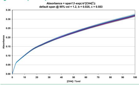
This NDIR methane sensor responds up to 100% methane but the housing is plastic so is not Ex approved.
